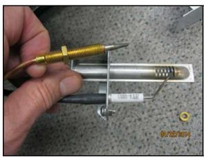
5. Begin removing the front bottom plate to gain access to the thermocouple and valve.
