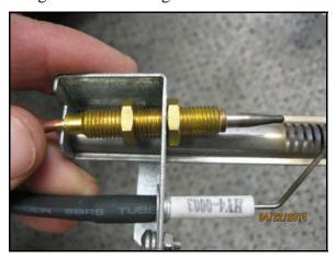
1. Positioning the tip as indicated, three slots in from the left of the bracket. Then tighten nuts.
