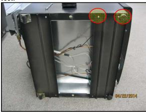
12. Replace the outer burner box cover. Before replacing the small viewing plate test fire the appliance to make sure the flame looks good and its align correctly under the boiler tube. Test to make sure the fridge stays running after you have released the gas button.
