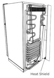
**Note: DO NOT install the appliance directly on carpeting.** Carpeting must be removed or protected by a metal or wood panel beneath the appliance, which extends at least the full width and depth of the appliance.
