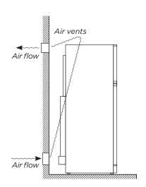
Fig. 4 Air flow - to release heat trap
