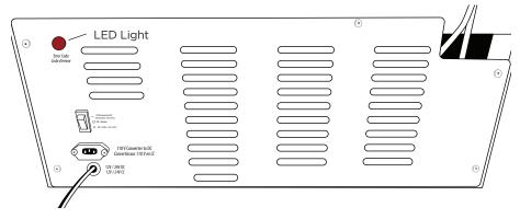
Remove screws from back plate to access the 15A in-line fuse, water catch basin, and compressor compartment
