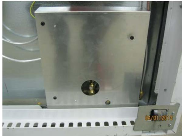
9. Before we stand the fridge up, locate the capillary, unravel and run up the side of the fridge to where the hole is located for entry to the into the cabinet
