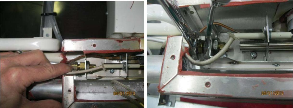
13. Disconnect the gas inlet line from the back of the inlet fitting, ensure to use a back up wrench
