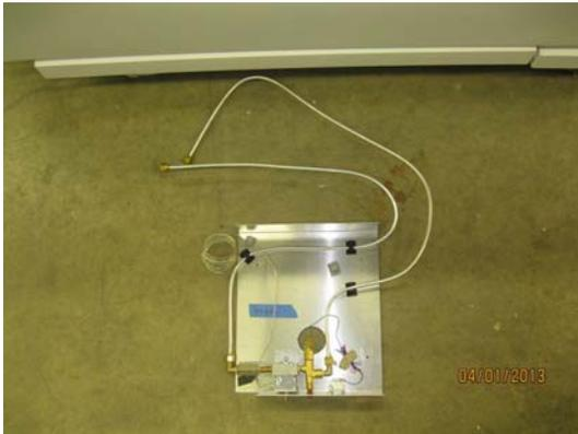
2. Attach the piezo and nut to the new plate and assemble the interrupter body into the back of the safety valve ensuring that you reattach the blue wire from the flame indicator to the spade on the block
