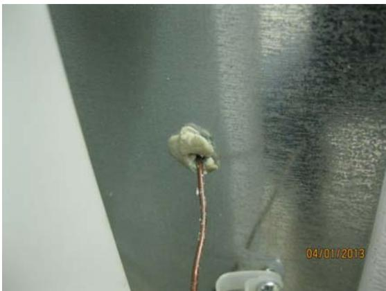
8. Pull the capillary tube out from the back of the fridge
