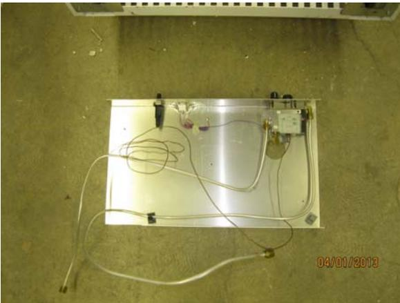
20. We now need to remove a few components from the old assembly to be used on the new assembly
