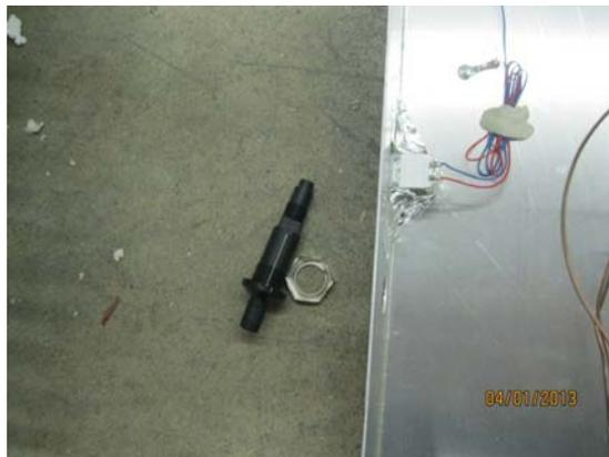
22. Unhook the blue wire from the interrupter block and remove the block to be used on the new assembly.
