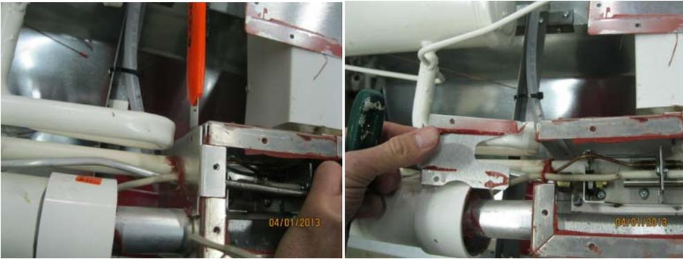
12. Disconnect the gas outlet tube from the orifice ensuring to use a back up wrench as shown
