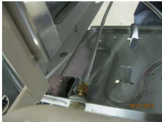
6. Reattach the outlet line to the orifice
