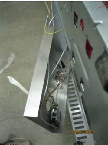
16. Unhook the piezo wire from the clip that may be holding it in place to the bottom of the plate
