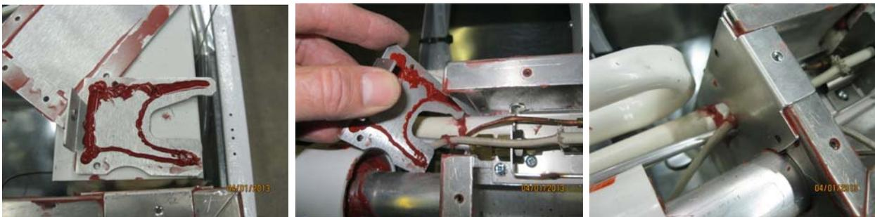
20. You will see that there is a gap that will need to be filled in with silicone. With the silicone tube provided, squeeze an required amount of silicone to fill the hole, now using two fingers, one from the inside of the box and one on the out side manipulate the silicone until the hole is filled.
